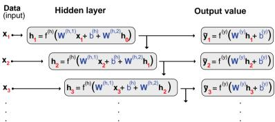
The first instance impacts all the network; the last instance impacts only the last layer. **Problem**: the successive iterations of the activation function yield vanishing gradients.
