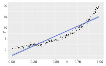
The error terms must have zero mean at any location of X. If not, errors may be correlated with X!
